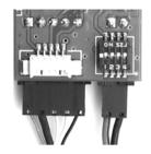
WARNING: DO NOT POWER TRANSMITTER WITHOUT ANTENNA ATTACHED. NO ANTENNA LOAD WILL DESTROY RF AMPLIFIER – NOT COVERED BY WARRANTY Small white connector on back of transmitter is for ImmersionRC Tiny Telemetry. See accessories.
