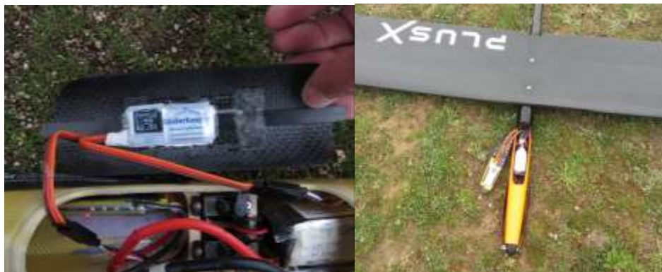
Glued installation in a Supra and Double side tape installation in a PlusX
